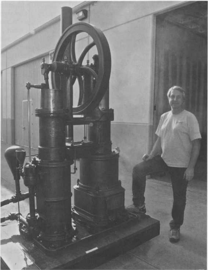
A RESTORED 8-INCH RIDER ENGINE VERY SIMILAR TO KIPLING'S
